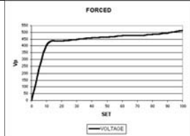
Diagrams of FORCED maximum mains voltage output versus Vp
